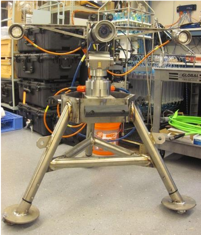
Above – Tripod equipped with Kongsberg Underwater Digital Stills Camera System with pan and tilt. Right – Tripod adjusted to full height
